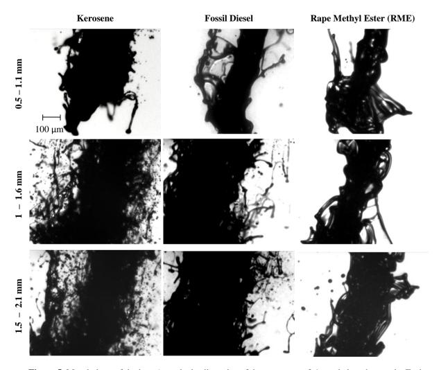
**Figure 5.** Morphology of the jet at/near the leading edge of the spray up to 2.1 mm below the nozzle. Each row represents the same spatial location.40 MPa injection pressure sprayed into atmospheric conditions.
