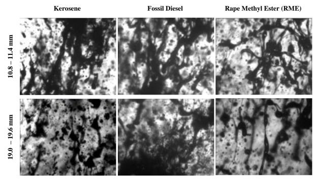
**Figure 7.** Morphology of the jet behind the leading edge of the spray at 10.8 mm (top row) and 19 mm below the nozzle (bottom row). Injection pressure of 40 MPa sprayed into atmospheric conditions.
