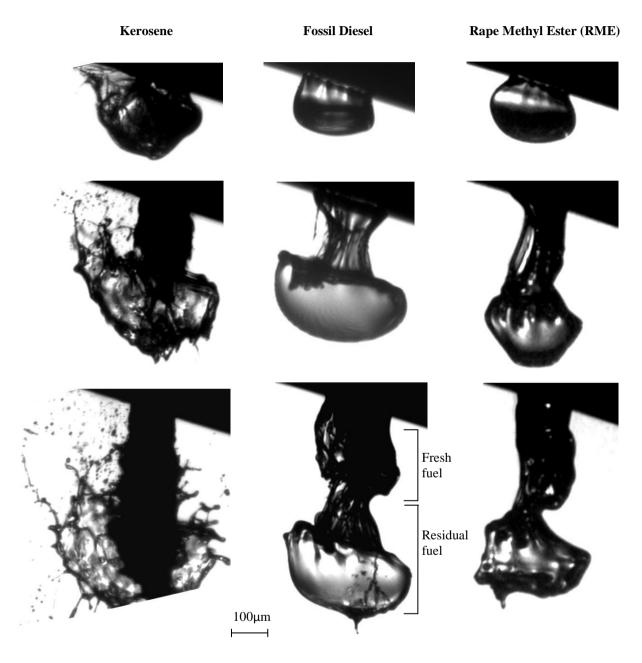
Figure 1. Initial jet formation during the SOI at 40 MPa injection pressure sprayed into atmospheric conditions.
